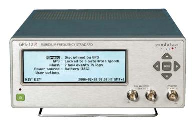
The Pendulum GPS-12R Portable Reference clock is an ultra-stable GPS-disciplined Rubidium reference, targeted for telecommunications application. Its high stability and low noise output, makes GPS-12R the ideal reference source for telecom instrumentation and testers, like SDH/PDH/Sonet Analyzers. Its Cesium standard performance, when locked to GPS, makes GPS-12R an ideal calibrator for metrology and test systems.
